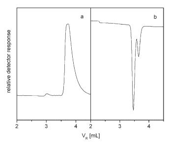
**Figure 4.** The chromatograms of toluene (a) and methanol (b) excess (30  $\mu$ L in 1 mL of eluent) injected into the tandem of two monoliths flushed with eluent toluene/methanol containing 85 wt. % of toluene.
