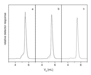
**Figure 10.** The LC LCI chromatograms of ultra-high molar mass polystyrene with M 30,000,000 g  $\cdot$  mol $^{-1}$ . Eluent was a mixture of toluene/methanol containing 85 wt. % of toluene. Sample volume  $v_i$  and sample concentration  $c_i$  were 50  $\mu$ L and 1 mg  $\cdot$  mL $^{-1}$ , respectively. 500  $\mu$ L barriers of toluene/methanol contained (a) (—) 30; (---) 40; (b) (—) 50; (---) 60 and (c) (—) 70 wt. % of toluene.
