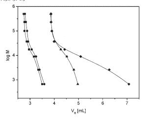
Figure 1. The log M vs.  $V_R$  dependences for polystyrenes in toluene. Tandem of two monoliths: ( $\blacksquare$ ) sample injected directly into column; ( $\bullet$ ) sample injected thru the barrier loop filled with eluent. ( $\triangle$ ) Tandem of three monoliths. For comparison also the values are shown, ( $\bullet$ ) obtained with the Kromasil 100A particulate column packing. M data are in g·mol<sup>-1</sup>.
