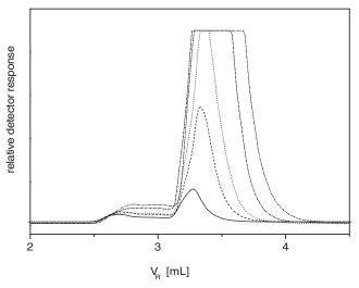
**Figure 5.** The LC LCI chromatograms for various injected concentrations  $c_i$  of broad polystyrene with mixed eluent toluene/methanol containing 85 wt. % of toluene. Injected volume  $v_i$  was 20  $\mu$ L, volume of barrier of neat methanol was 100  $\mu$ L. Injected concentrations were: (—) 2; (---) 5; (. . . .) 10; (-.--) 25 and (-.---) 50 mg·mL<sup>-1</sup>.
