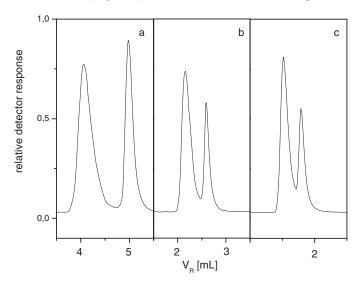
**Figure 7.** The LC LCI chromatograms of a mixture of broad PS plus PMMA with molar mass 103,000 g  $\cdot$  mol<sup>-1</sup>, 1 mg  $\cdot$  mL<sup>-1</sup> each. Injected volume was 50 μL. Tandem of three monoliths, eluent was toluene/methanol containing 85 wt. % of toluene. 100 μL barrier of toluene/methanol mixture contained 20 wt. % of toluene. Flow rates: (a) 1 mL  $\cdot$  min<sup>-1</sup>; (b) 2 mL  $\cdot$  min<sup>-1</sup>; (c) 3 mL  $\cdot$  min<sup>-1</sup>.
