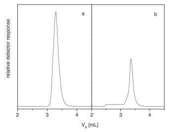
**Figure 15.** The LC LCI chromatograms of polystyrenes eluted from a tandem of two monoliths. Eluent was a mixture of toluene/ACN containing 50 wt. % of toluene. Sample concentration  $c_i$  and sample volume  $v_i$  was 1 mg  $\cdot$  mL<sup>-1</sup> and 20  $\mu$ L, respectively. Barrier was 100  $\mu$ L of neat ACN. Molar masses of PS: (a) 2,600 and (b) 498,000 g  $\cdot$  mol<sup>-1</sup>.
