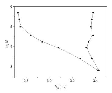
Figure 14. The log M vs.  $V_R$  dependences for polystyrenes with a tandem of two monoliths and mixed eluent toluene/ acetonitrile containing 50 wt. % of toluene. Sample volume  $v_i$  and sample concentration  $c_i$  were 20  $\mu$ L and 1 mg·mL $^{-1}$ , respectively. ( $\blacksquare$ ) sample without barrier ( $\blacksquare$ ) sample with a 100  $\mu$ L barrier of neat ACN.
