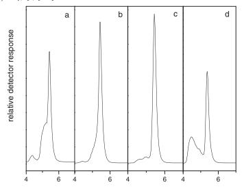
Figure 11. The LC LCI chromatograms of broad polystyrene. Eluent was a mixture of toluene/methanol containing 85 wt. % of toluene. Sample volume  $v_i$  and sample concentration  $c_i$  were 50  $\mu$ L and 1 mg  $\cdot$  mL<sup>-1</sup>, respectively. The barriers of toluene and methanol were applied containing: (a) 30; (b) 50; (c) 60 and (d) 70 wt. % of toluene.
