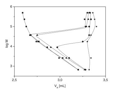
Figure 12. The log M vs.  $V_R$  dependences for polystyrenes dissolved and injected in pure toluene into a tandem of two monoliths columns. Injected volume  $v_i$  and injected concentration  $c_i$  were 50  $\mu$ L and 1 mg · mL $^{-1}$ , respectively. Eluents were mixtures of toluene/methanol containing ( $\square$ ) 80; ( $\bullet$ ) 70; ( $\blacktriangle$ ) 65; ( $\bullet$ ) 57; and ( $\bigstar$ ) 54 wt. % of toluene.
