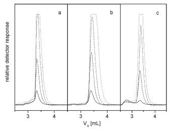
Figure 2. The typical LC LCI chromatograms for a set of two monoliths monitored with toluene/methanol eluent containing 85 wt. % of toluene and with 100 μL barrier of neat methanol. Injected volumes  $v_i$  were (—) 20 μL; (-..-) 50 μL; (----) 100 μL and (....) 200 μL. Molar masses of polystyrene (a) 9,000; (b) 498,000; (c) broad molar mass sample with  $\overline{M}_w = 180,000$  and  $\overline{M}_n = 67,000$  – all data are in  $g \cdot mol^{-1}$ .
