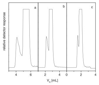
Figure 8. The LC LCI chromatograms of a mixture of broad PS plus PMMA with molar mass 103,000 g·mol $^{-1}$ . Injected solution contained 0.1 g of PS and 1 mg of PMMA in 1 mL. Injected volume 50  $\mu$ L. Eluent toluene/methanol contained 85 wt. % of toluene. 100  $\mu$ L barrier of toluene/methanol contained 20 wt. % of toluene. Flow rates: (a) 1 mL·min $^{-1}$ ; (b) 2 mL·min $^{-1}$ ; (c) 3 mL·min $^{-1}$ .
