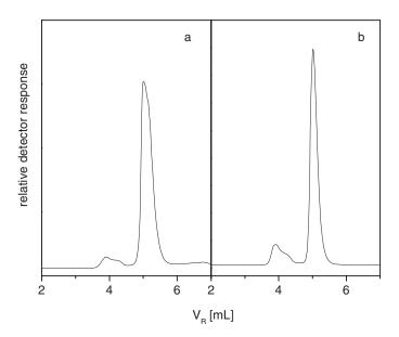
**Figure 9.** The LC LCI chromatograms of ultra-high molar mass polystyrenes with M: (a) 20,600,000 and (b) 30,000,000 g  $\cdot$  mol<sup>-1</sup>. Eluent was a mixture of toluene/methanol containing 85 wt. % of toluene. Sample volume  $v_i$  and concentration  $c_i$  were 50 μL and 1 mg  $\cdot$  mL<sup>-1</sup>, respectively. 100 μL barrier of toluene/methanol contained 20 wt. % of toluene.
